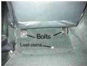
Slide the seat all the way forward, and tilt the seat back forward. You should see the bolts in the back of the two seat tracks. Remove these bolts with your 14mm socket.
