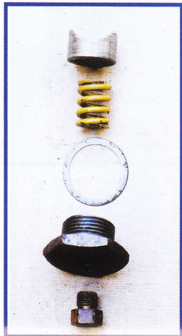
Fig 9 From left to right: grease plug, cap nut, shim, spring, and plunger assembling to the housing, until you can only just detect pinion movement. Any movement is easier to detect if no
