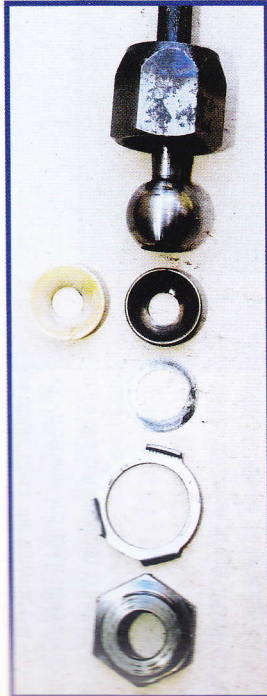
Fig 10 From left to right: sleeve nut, tab washer, shim, cup (steel or plastic), track rod, cup nut
