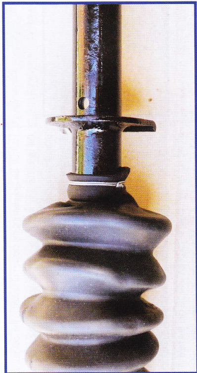
Fig 12 Locating hole for nylon button With a little use and as more grease is worked into the ball and
